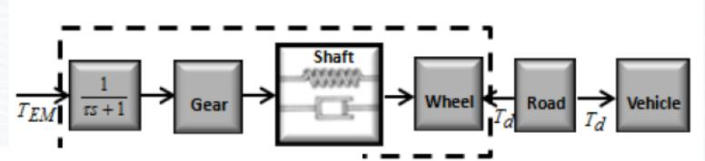
$$\begin{pmatrix} \dot{\theta}_{motor} \\ \dot{\theta}_{motor} \\ \dot{\theta}_{wheel} \\ \dot{\theta}_{wheel} \\ \dot{T}_{EM} \end{pmatrix} = \dot{\mathbf{x}}_s = \mathbf{A}_s \mathbf{x}_s + \mathbf{B}_s T_{dem}$$
