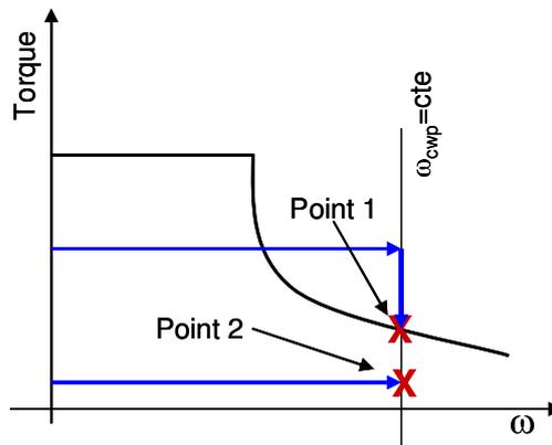
**Fig 3** Checking the value of the required braking torque in the working point
