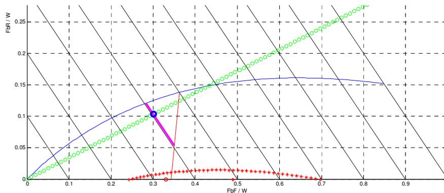
**Fig 1** Representation of the braking calculations with friction limit
