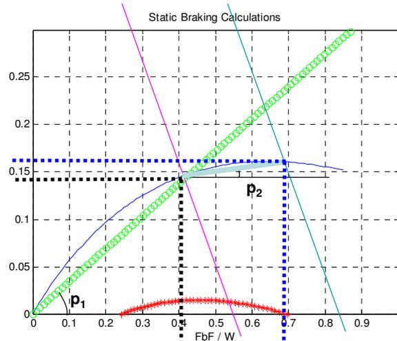
Fig 2 Braking force distribution of bilinear strategy
